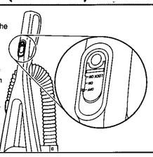
3 To stop the vacuum cleaner, pull the switch on the handle to the OFF position
