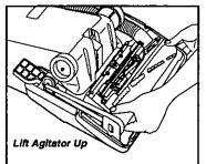
Remove the agitator brush assembly, (carefully lift it out), and remove the worn or broken belt from the agitator pulley and motor shaft
