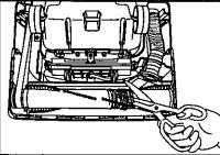
Switch off the vacuum cleaner and unplug the power cord before cleaning the agitator assembly In order to keep the cleaning efficiency high, clean the agitator assembly regularly Remove the lower plate if necessary See the REMOVING/INSTALLING THE LOWER PLATE section for the proper procedure
