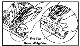
After checking the end caps, reinstall the agitator brush assembly back into the housing grooves After installing the agitator brush assembly, turn it by hand making sure that the belt is not twisted or pinched and all rotating parts turn freely Replace the lower plate as described in the REMOVING/INSTALLING THE LOWER PLATE section
